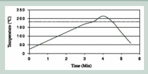
This profile is designed for use with Sn63/Pb37 and Sn62/Pb36/Ag2 and can serve as a general guideline in establishing a reflow profile for use with other alloys. Adjustments to this profile may be necessary based on specific process requirements.
