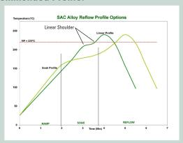
The stated profile recommendations apply to most Pb-free alloys in the SnAgCu (SAC) alloy system, including SAC305 (96.5Sn/3.0Ag/0.5Cu). This can be used as a general guideline in establishing a reflow profile when using Indium10.1 solder paste. Deviations from these recommendations are acceptable, and may be necessary, based on specific process requirements, including board size, thickness, and density. Start with the linear profile, then move to the optional soak profile if needed.
