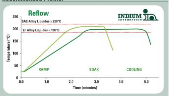
This profile is designed for use with **Durafuse™ LT** in Indium5.7LT-1. This can be used as a general guideline in establishing a reflow profile for **Durafuse™ LT** Solder Paste. Deviations from these recommendations are acceptable, and may be necessary, based on specific process requirements.
